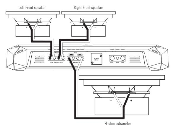
2-channel (bridged) operation: Connect one speaker's + lead to the Front L+ terminal, and the - lead to the Front R- terminal. Connect the other speaker's + lead to the Rear L+ terminal, and the - lead to the Rear R- terminal.
