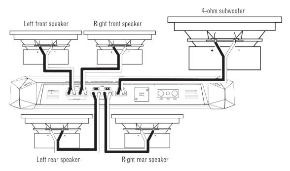
3-channel (front and rear bridged) operation: Connect one speaker's + lead to the Front L+ terminal, and the - lead to the Front R- terminal. Connect the other speaker's + lead to the Rear L+ terminal, and the - lead to the Rear R- terminal. Connect the subwoofer's positive (+) lead to the + terminal, and the negative (-) lead to the - terminal.
