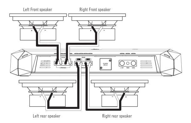
• 3-channel operation: Connect the stereo speakers to the Front terminals, as described above. Connect the single speaker's + lead to the Rear L+ terminal, and the - lead to the Rear R- terminal.
