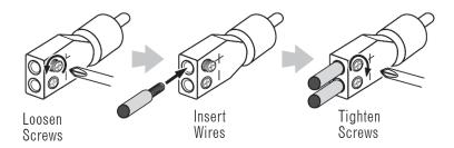
Always connect the (+) speaker wire to the adapter's (+) terminal and the (-) speaker wire to the adapter's (-) terminal. When all wires are connected, plug the adapters into the Club amplifier's FRONT (and REAR, if using the 4-channel amplifier) preamp inputs.
